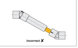
In extensible transmissions make sure that the arrows are perfectly aligned.
