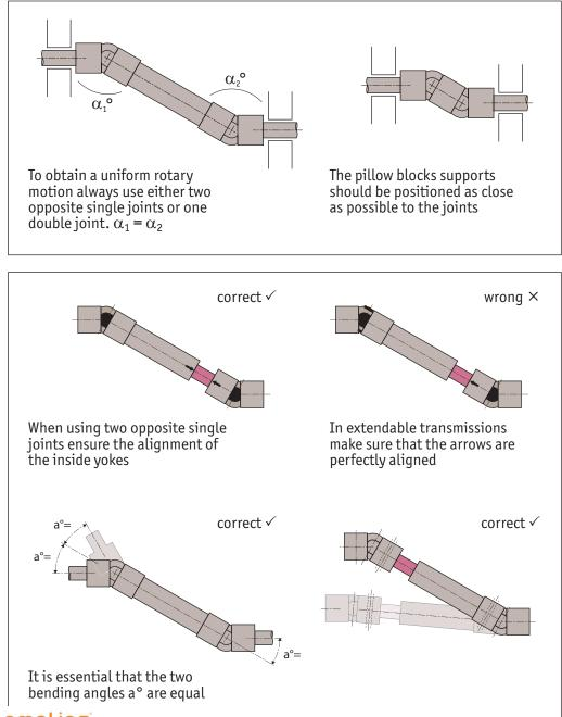
iversal Joints from Automotion Components
