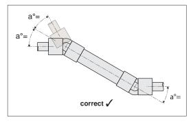
It is essential that the two bending angles a° are equal.
