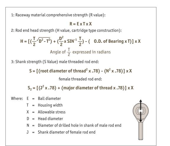
The axial static load capacity is measured as the force required to cause failure via a load parallel to the axis of the bore. Depending on the material types and construction methods, the ultimate axial load is generally 10-20% of the ultimate radial static load. The formula does not account for the bending of the shank due to a moment of force, nor the strength of the stake in cartridge-type construction.
