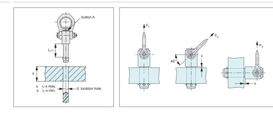
Note: The full shaft must be engaged. Longer shaft lengths
