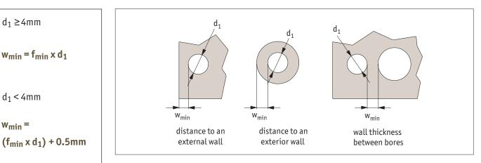
The quidelines for minimum wall thickness or distance from and edge (Wmin) are shown below – these minimum values produce only a very slight deformation on the exterior profile (less than 20 microns).
