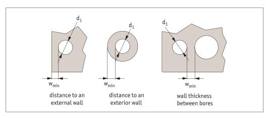
The guidelines for minimum wall thickness or distance from and edge ( $W_{min}$ ) are shown below – these minimum values produce only a very slight deformation on the exterior profile (less than 20 microns).
