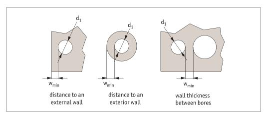
The guidelines for minimum wall thickness or distance from and edge ( $W_{min}$ ) are shown below – these minimum values produce only a very slight deformation on the exterior profile (less than 20 microns).
