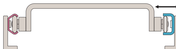
T and U rail allows for misalignment
