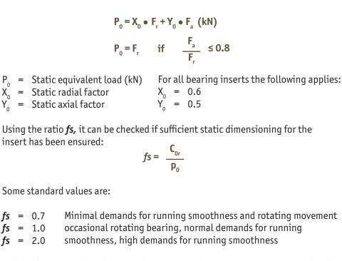
For situations where there are radial and axial loads on the static or slow moving bearings:
