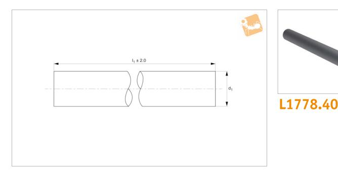
Aluminium EN AW 6061/6060 Surface: Hard anodized Hardness: 450-550 HV
