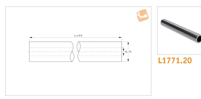
Carbon steel (C60), surface hardness 60-65 HRC. Surface finish  $0.3-0.6\mu$  Ra, ground and polished to 8-12 cla.
