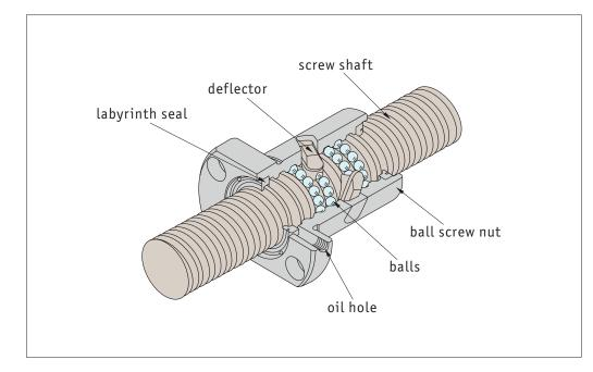
Lubrication - the ball screws must be adequately lubricated. This is dependent on load, speed, motion sequence and temperature. Do not use lubricants containing Mo/So or graphite.
