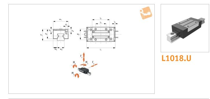
Aluminium block (X46Cr13 hardened to F35), tensile strength 350N/mm<sup>2</sup>. Stainless steel inserts hardened, and stainless ball bearings (DIN 1.4034).
