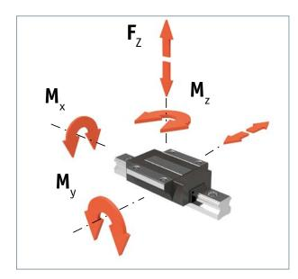
Calculation of load on bearing for a carriage:
