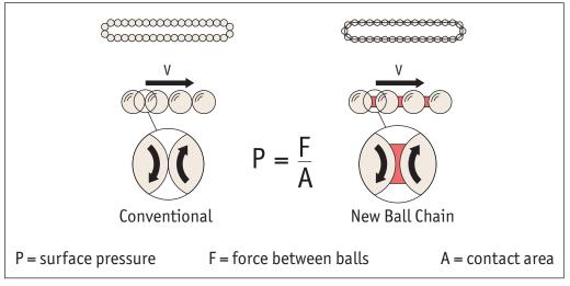
The rotating balls in conventional profile rail guides have point contact between each other. The rotation speed at the contact point is double the speed of the balls. The contact area (A) is so small that the surface pressure (P) tends towards infinity. This leads to heating and wear of the balls and the linear guide system.
