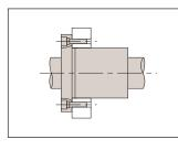
See part tolerances for perpendicularity accuracy  $\bot$  when outer sleeve is used as datum for installation.
