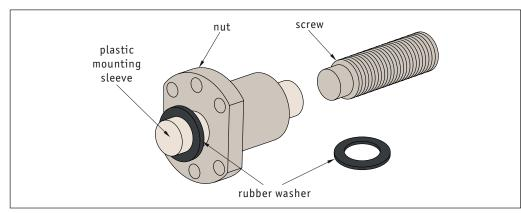
Ball nuts should be mounted only with the help of a plastic mounting sleeve (delivered with the nut). The start of the thread should be aligned so that the seal and the internal parts of the nut are not damaged.
