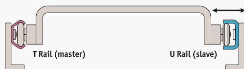
T AND U RAIL ALLOWS FOR MISALIGNMENT
